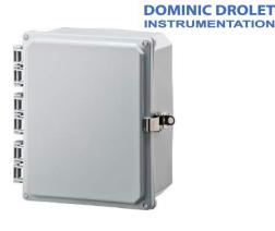
Integra polycarbonate enclosure, hinged and lockable lid, DIN rail and mounting kit included. Key Specifications: Temperature Range = -40 to 265 °F, Flame Rating = UL, 5VA. (Test Spec. UL-94), Outdoor UV Exposure = F1. (Test Spec UL), UL-50/c-UL Type 4X Listed (file #E207562) IP 66.
