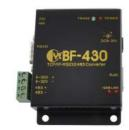
The RS485 to Ethernet Converter is a universal serial device server that enables users to connect Modbus RS485 sensors to the eGauge using a local area network. The BF430 requires a power supply (EA1001, page 8) or a direct +/- 9-30VDC connection for power.
